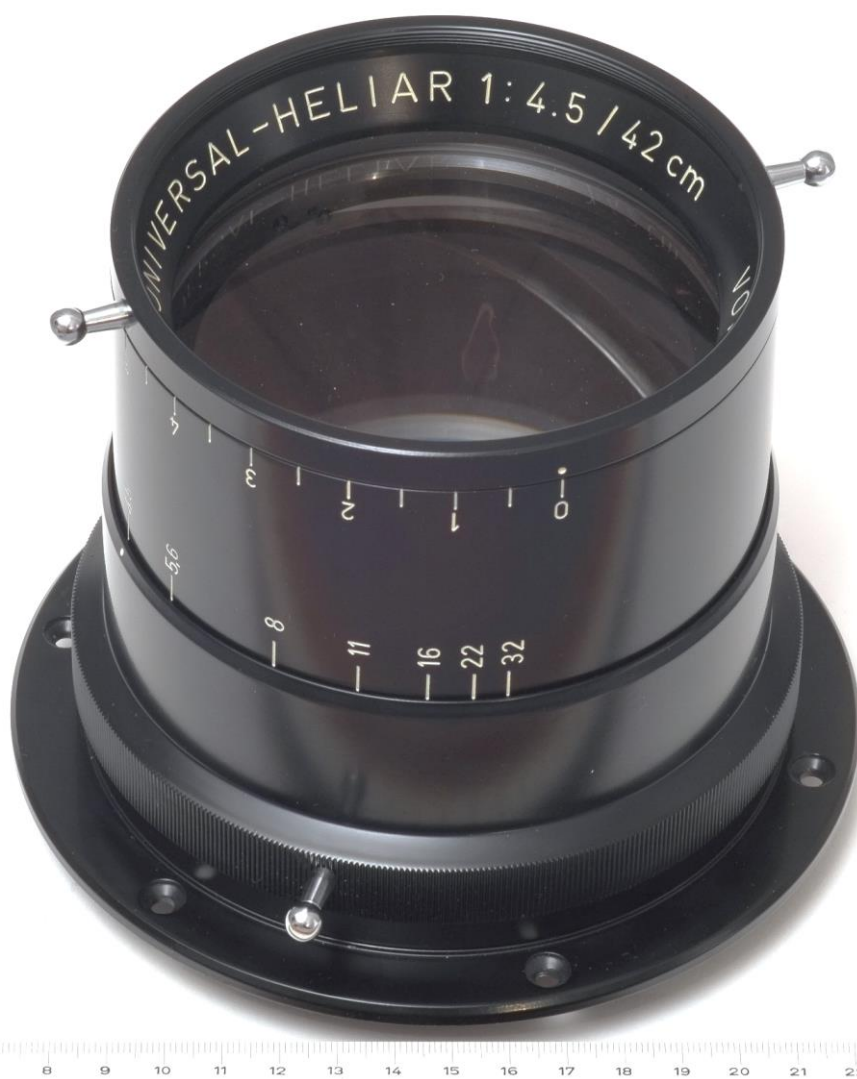
Fig. 5: Post-WW II Universal Heliar 420mm f/4.5. Apart from the coating and the inscription font, prewar and postwar versions can be distinguished by the shape of the “handles” for the aperture and the soft focus effect. Prewar handles are knurled, cylindrical, and nickel-plated, the postwar handles are smooth with a small ball at the end and chrome-plated, as shown above. The lower handle set changes the aperture, the one near the lens front changes the position of the central biconcave lens. The “0” setting shown above is without soft focus, the highest soft setting is “5”. Scale is in cm.
