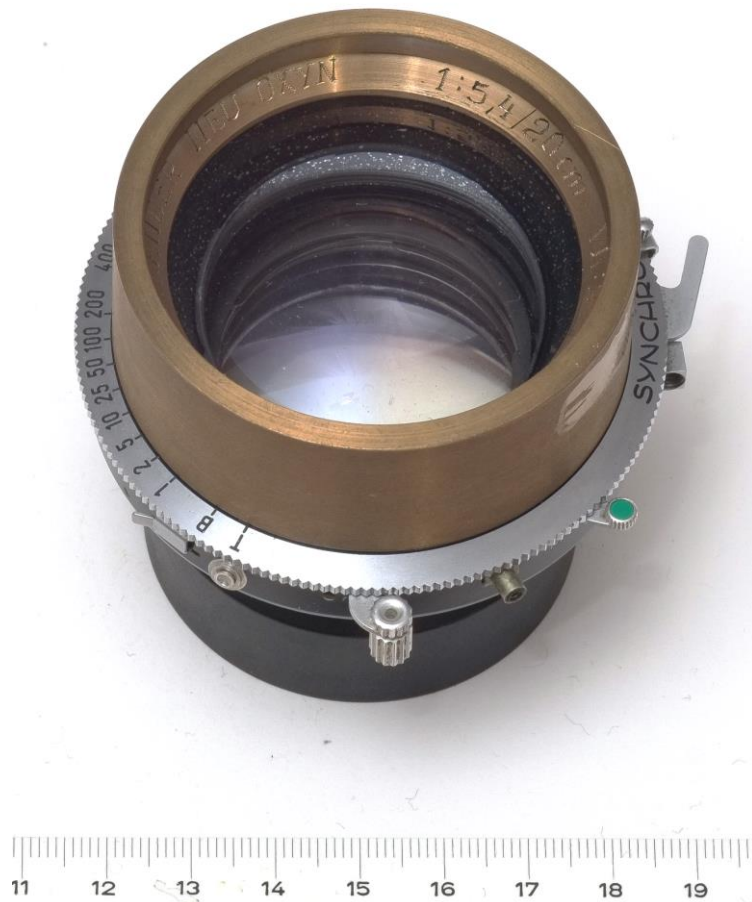
Fig. 11: “Neu-Oxyn” 200mm f/5.4 prototype lens by Voigtländer, a Plasmal type similar to the Symmar from Schneider-Kreuznach. Scale is in cm.
