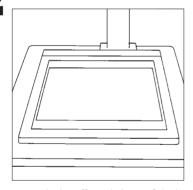
Switch the room light off and, by safelighting, position the easel under the enlarger to frame the print as you want it. Take out a new sheet of MULTIGRADE paper, and place this on the easel. Using the timer, give the paper the correct exposure worked out by examining the test print.
