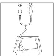
Wash the print for 2 minutes in a good flow of water ideally at about 20°C/68°F but cold water above 5°C/41°F will give adequate washing. Empty the wash tray a few times to ensure a complete change of wash water, or use rubber tubing to syphon water from the bottom of the tray.
