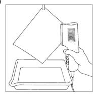
After the wash, drain the print and use a squeegee or sponge to remove any excess water. Attach a wooden or plastic clip to one corner, and hang the print over a drip tray to dry. Drying can be speeded up by using a hairdryer on a low setting, kept moving and about 30cm/1ft away from the print. MULTIGRADE prints dry naturally in a warm room in under 30 minutes.
