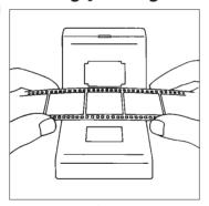
Choose the negative for printing, and make sure it is clean. Remove any dust with a puffer brush. Hold the negatives so you can read the edge numbers, then turn the negatives round (not over) so the numbers are furthest away from you. Place the negatives in the negative carrier of the enlarger. Slide the negative carrier into place. Switch on the safelight and switch off the roomlights.
