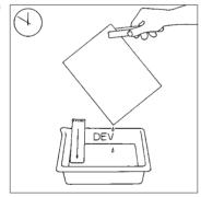
Check the thermometer in the dish of developer (20°C/68°F) and set the timer to zero. Slide the paper quickly and smoothly into the developer, making sure there are no air bubbles on the shiny surface. Start the timer. Rock the developer dish continuously backward and forward to send the solution gently over the print. After 50 seconds, use tongs to lift the paper out, and drain off the developer.
