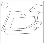
Slide the paper into the dish of fixer, and rock the dish to get a good flow of chemicals over the surface of the print. Fixing takes only 30 seconds in fresh solution. It does not matter if this time is exceeded slightly, but prints should not be left in the fixer for minutes on end. If not washing a print straight away, store it in a dish of clean water.
