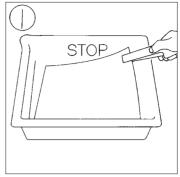
As one minute shows on the timer, quickly and smoothly slide the developed paper into the stop bath. take care not to contaminate the developer tongs with the stop bath. Rock the dish for about 30 seconds. Use the second pair of tongs (from the fixer) to lift the print while solution drains from it, and transfer it to the dish of ILFORD RAPID FIXER solution. (The timing of this step is not critical.)
