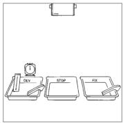
Set up your safelight (e.g. the ILFORD SL1 safelight) at least 1.2m/4ft from the developing dish. Lay out three processing dishes, label them DEV, STOP and FIX, two pairs of print tongs, and a clock for timing development. Then mix up the processing chemicals using water at about 23°C/73°F. The aim is to process at a working temperature of  $20^{\circ}\text{C}/68^{\circ}\text{F}$  +/-  $1^{\circ}\text{C}/2^{\circ}\text{F}$ , so a few degrees are allowed for heat lost in mixing and cooling.
