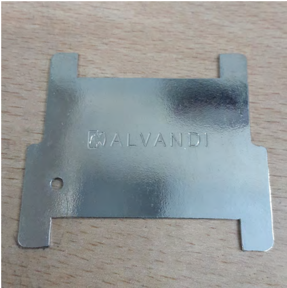
Exchange tool wrench for lens retaining rings 0/1 shutter
