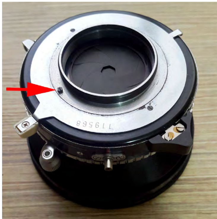
Remove the screw shown from the back of the shutter 0/1
