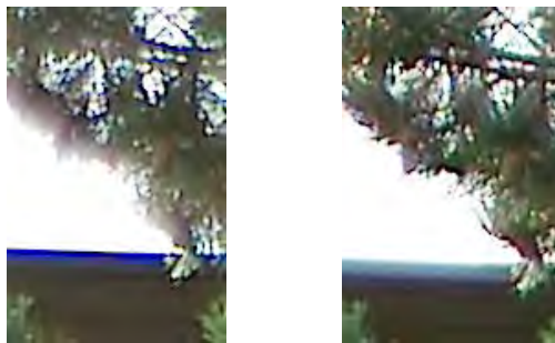
Images of two high-speed wide angle lenses at full aperture, details near the edge.
