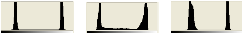
The characteristics of the images above are also illustrated by their histograms: In the picture of the lens with poor micro contrast (middle) the right peak in particular is broadened towards the left, because the white at the edges with glare lights up the areas which are in reality black. The separation of the two peaks on the gray scale is the same as with the good picture on the left, however.
