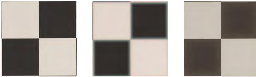
Enlargements of format-filling images of a chess board, left with perfect imaging quality, in the middle with low micro contrast, right with high degree of veiling glare.
