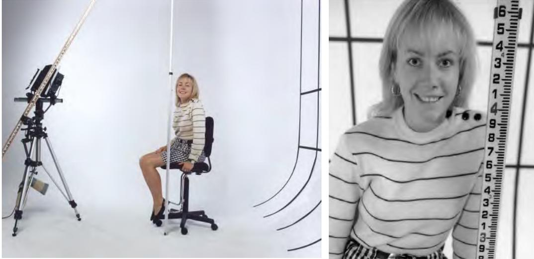
**Example 4 illustrates the hinge rule under quite different circumstances. 30° of back tilt combined with 26° of lens tilt (4° relative to the back) put the hinge line 7 feet from the lens and about 6 feet directly over the subject's head. Focusing with the camera back now causes the plane of sharpest focus to swing from the hinge line like a pendulum. The result is distorted, but in focus.**
