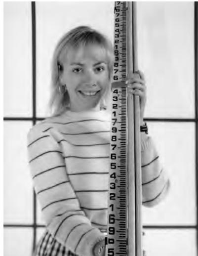
**Example 2:** The survey rod was raised to a higher angular position and the camera back moved away from the lens to focus on the rod in this new position. Again the rod is in focus from end to end. So long as the rod remains hinged at a point 4.2 feet directly below the lens, 7° of lens tilt is the amount required to focus on the rod at any angular position.
