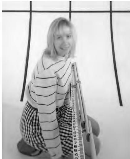
**Example 3:** The vertical portion of the rod was raised to put the hinge just over 2 feet below the lens. The required amount of lens tilt is now 14°. The camera will again focus on the whole rod, even when it is angled away from the camera.
