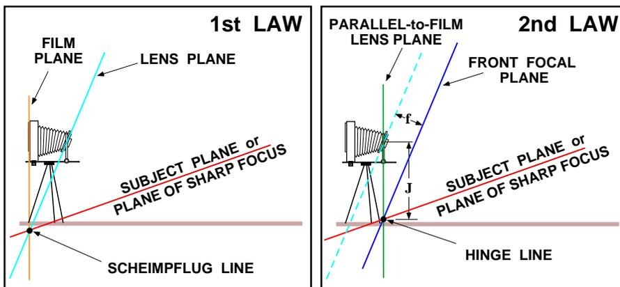
The First Law of the view camera—the Scheimpflug Principle—requires that the Film Plane, the Lens Plane and the Subject Plane must intersect along a single line. In this side view the line is seen as a dot.
