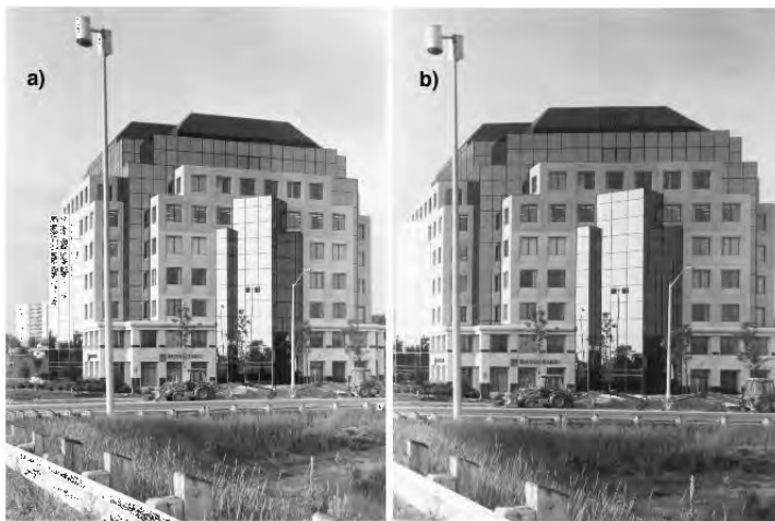
Figure 6: a) shows a ‘correct’ image of a building. Front rise only was used for this photo. In b) the back was swung by almost 40^\circ to give a rather odd and ‘incorrect’ image. This second photo looks in some ways as though it was taken from a camera position to the photographer’s right. But other clues indicate this is not the case: we can see the left side of the building, for example, and we know that most buildings have 90^\circ corners. Swinging the back also stretches the image horizontally.
