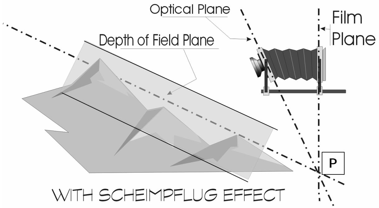
Note that all planes intersect at a point (P). In fact, the depth of the plane encompassing the Depth of Field has not been increased at all, it has merely been tilted so that it coincides with the intended subject matter.
