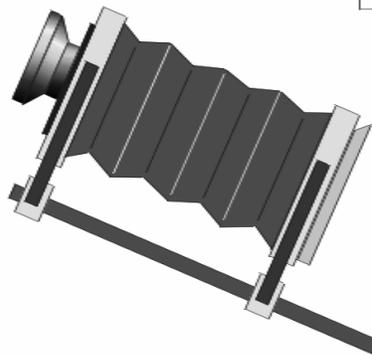
With the Film Plane at an angle to the object, those parts of the object farther away look smaller. However it is often desirable to avoid this forced perspective.
