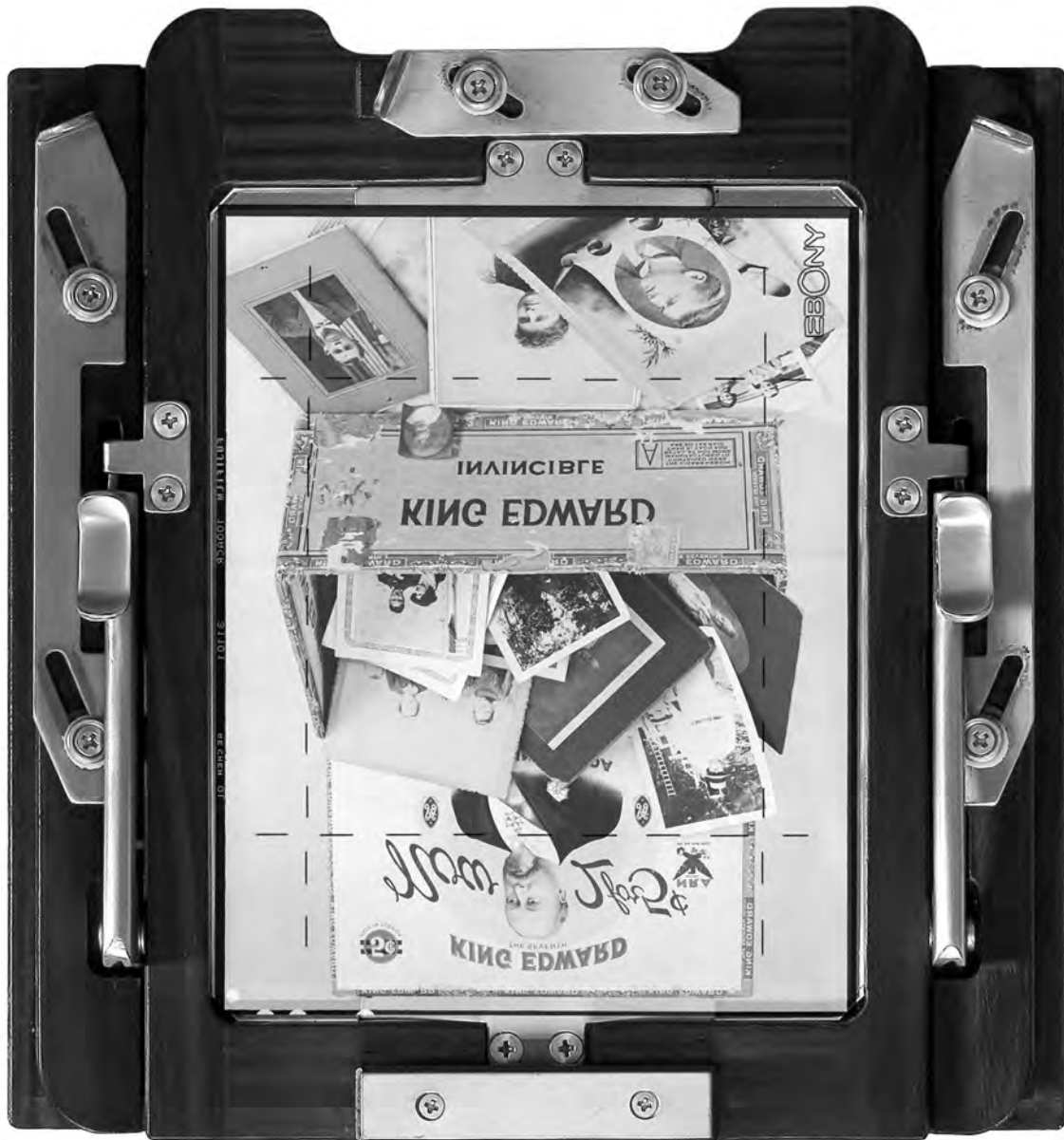
superimposed transparency indicating position of asymmetrical pivot marks relative to image as it appears on focusing screen
