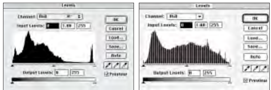
Figure 1. Here we see two histograms. The first is from a good scan without manipulation in Adobe Photoshop. Notice that there is data running from each end of the tonal scale (0 to 255) and that the histogram is solid black, meaning we captured good data throughout. The second histogram came from a poor scan that lacked tonal data from either end of the scale. Using Photoshop, the tonal deficiencies were corrected with the Levels tools. Notice the resulting histogram has a combination effect, in which each white step represents data loss.
