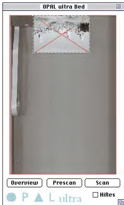
Figure 6. This is a screen dump showing the prescan of the bed of a Linotype Opal Ultra tabloid sized scanner. Notice that I have the long axis of the original placed on the scanner bed in a direction opposite from the way the CCD moves up and down the bed. This means that the CCD travels over a shorter area of the scanner, which can speed up scanning.
