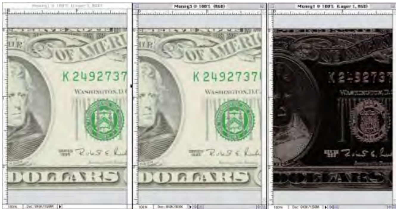
Figure 7. The two scans of the $20 bill should appear identical. But notice the third image, which is the two images on one layer with the Difference mode applied. You can see the subtle lines, which illustrate the minor differences between the two scans.
