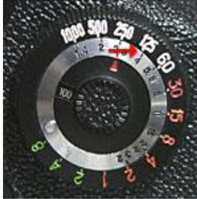
Similarly, by looking at the dial, you can quickly see that 1/60 second at F5.6, 1/30 second at F8 or 1/15 second at F11, etc. will also work. If the numbers don't line up exactly, you can always set the lens to a half stop setting (if possible), or just use your judgment and select an exposure that you think will work for the scene in front of you.
